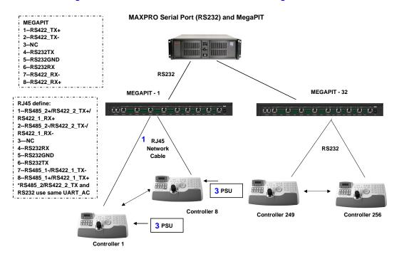
PORTS 1 RJ45 define: 1--RS485 2+/RS422 2 TX+/ RS422 1 RX+ 2--RS485\_2-/RS422\_2\_TX-/ RS422\_1\_RX-3-NC 4--RS232RX MX18 TX DATA 4 SIGNAL GROUND 5--RS232GND 5 MX18 RX DATA 6--RS232TX 7--RS485\_1-/RS422\_1\_TX-8--RS485\_1+/RS422\_1\_TX+
